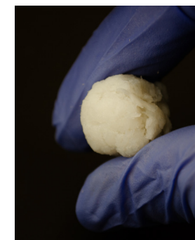
NMP Fibers after hydration with water
